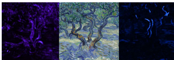
Fig. 7. Element maps for cobalt (left) and iron (right). Detail of the central tree of Olive Trees (center). The elemental maps show the use of cobalt blue to define the central and right tree trunks in the early stages of painting, followed by final outlining strokes of Prussian blue that modify the central trunk.
