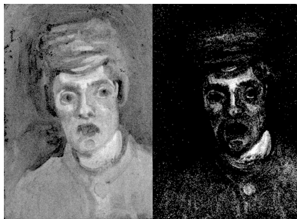
Fig. 13. Elemental map showing the antimony distribution near the surface (left) and at depth (right), Head of a Man (1885)
