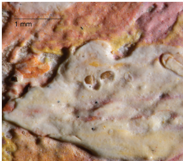
Fig. 6. Photomicrograph of sand found in the paint layer of Study for "The Channel of Gravelines, Petit Fort Philippe" (1890)
