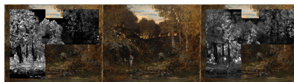
Fig. 17. A: the distribution of arsenic in the areas mapped by MA-XRF, corresponding to emerald green that surrounds the negative spaces occupied by trees on the left of the composition; B: visual appearance of the painting for comparison; C: the distribution of chromium, corresponding to viridian, chrome yellow, and zinc yellow, which also define negative spaces occupied by the former trees. The Eagle's Nest, Forest of Fontainebleau (ca. 1837–67)
