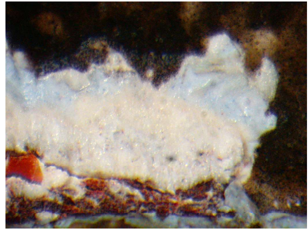
Fig. 20. Photomicrograph of Exit from the Theater (after 1863), showing sky blue paint from the underlying landscape and its ground layer exposed at an edge loss, field of view is approximately 0.5mm
